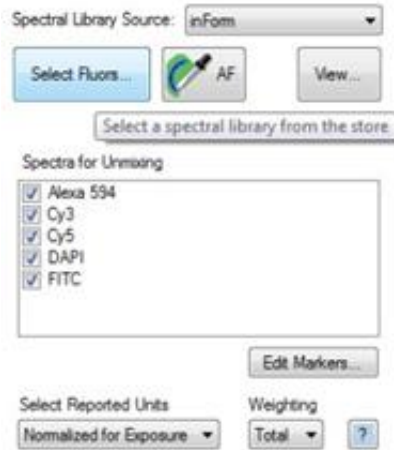
FIGURE 8.2. Selecting inForm as the Spectral Library Source to choose spectra that were created in inForm.
